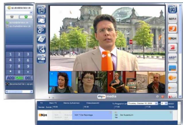
Figure 1 Client of the Interactive Television System, showing a main TV channel and four on-screen displays at the bottom.
