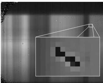
Fig. 5. Defect pixels in a hyperspectral image.
