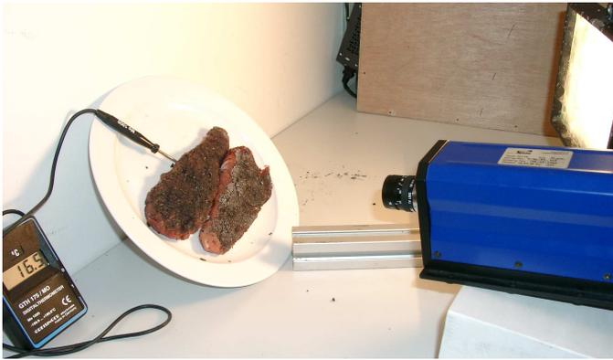
Fig. 8. Experimental set-up, here: pork with a layer of coal ash.
