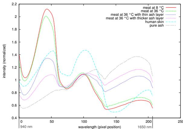
Fig. 9. NIR spectra of meat at different temperatures and ash layers and spectra of skin in comparison.
