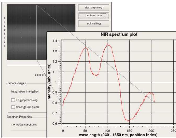
Fig. 4. A hyperspectral image and the plot of one spectrum.
