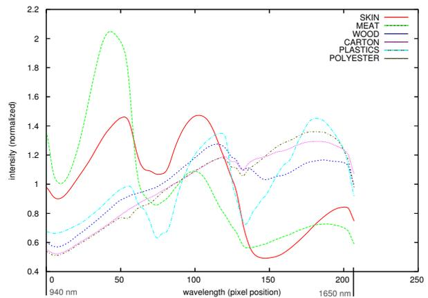
Fig. 7. The reference spectra used to calculate the spectral angle of a sample spectrum.
