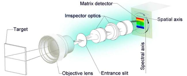
Fig. 3. Principle of the line scan camera ImSpector N17E, courtesy of Specim.
