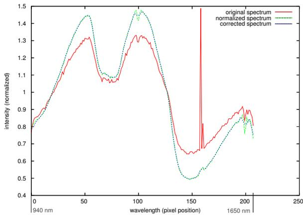
Fig. 6. Spectrum plot. First curve: spectrum in original image; second curve: spectrum after defect pixel correction and normalization; third curve: spectrum after all preprocessing steps.
